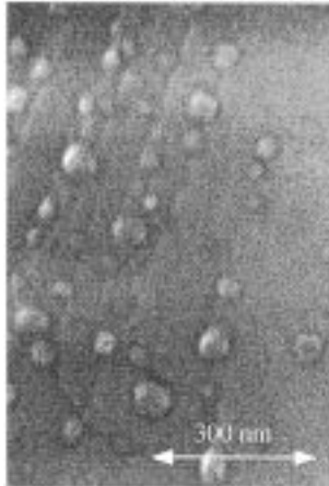
Fig.5 SEM image of 3C-SiC epilayer surface by APCVD. Flow rate of SiH 4 : 0.8 sccm, C 3 H 8 : 0.6 sccm and H 2 : 8 slm.
