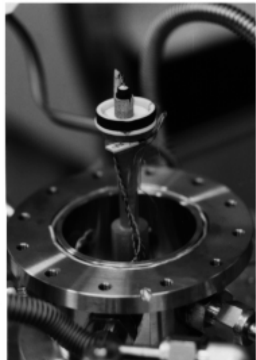
Fig.2 Photograph of Bi 2 Sr 2 CaCu 2 O x sample set at the sample holder of the apparatus
