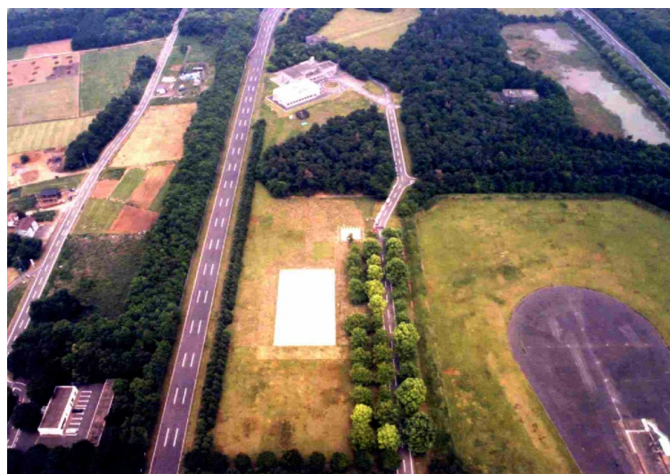
Photo 1 ETL open-area site for antenna measurement and the circumstance around the ground plane in the AIST second research center. A white large rectangle is the ground plane. A smaller one at the upper and right hand side is the top of the underground measurement room. The nearest objects to the ground plane on the ground are three lines of trees at the right hand side. There is a road for automobile test-run at the opposite side. This photo is offered by Advanced Engineering Service
