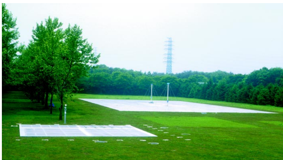
Photo2 ETL Open area antenna site
