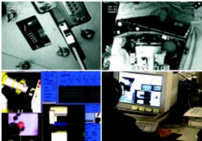
Fig.18 Operation scene in remote teaching (Top left: Taskboard view through hand-eye camera, Top right: Hand and taskboard view through monitor camera, Bottom left: Superimposed display of 3-D CG and real video image, Bottom right: Operator console)
