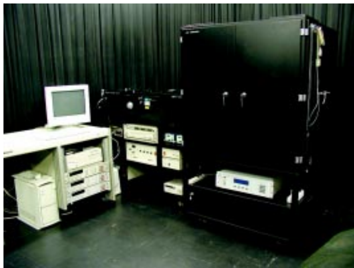
Fig.4 Spectral responsivity calibration system
