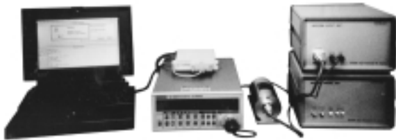
Figure 8.2 Front view of the measurement system. A laptop PC is used as a system-controller.
